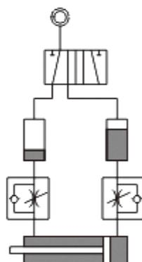
Air/Oil systems combine the speed and low cost of air operation with the smooth, even actuator control of oil from a standard air line source.
